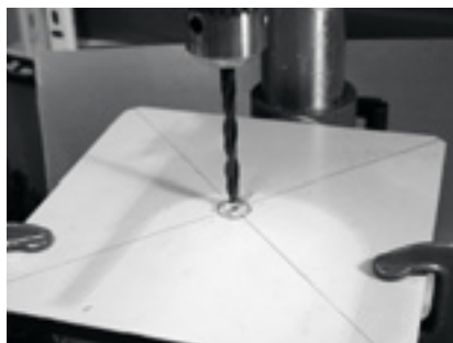
Figure 4.21: Drilling the hole in the metal plate.
