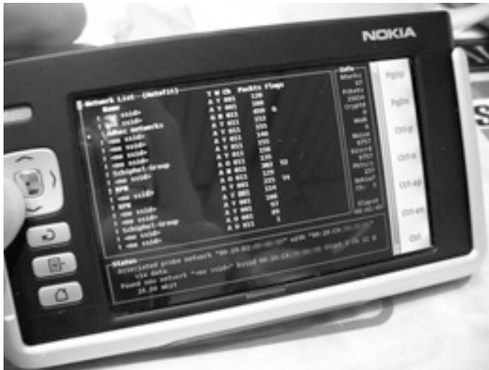
Figure 6.12: Kismet running on a Nokia 770 Internet Tablet
