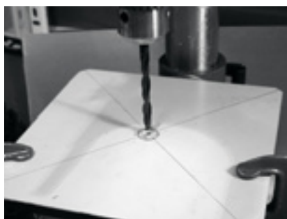
Figure 4.21: Drilling the hole in the metal plate.
