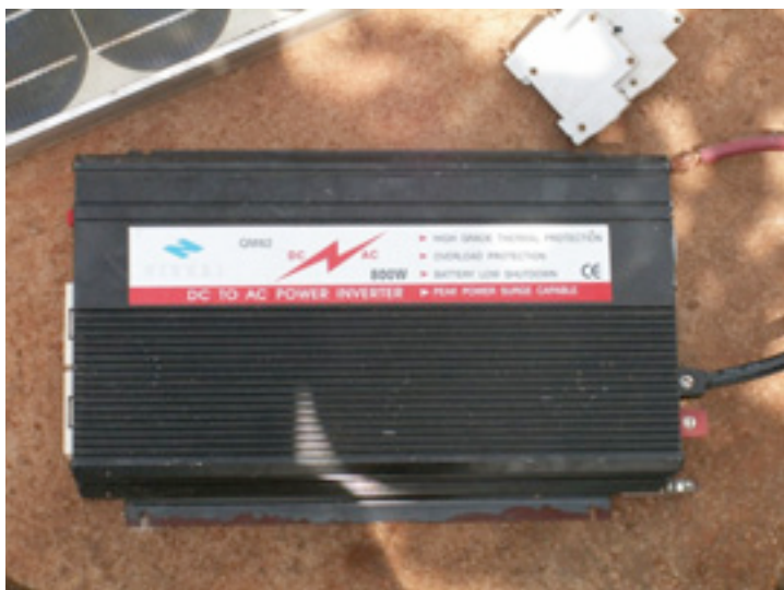
Figure 7.4: An 800 Watt DC/AC converter (power inverter)
